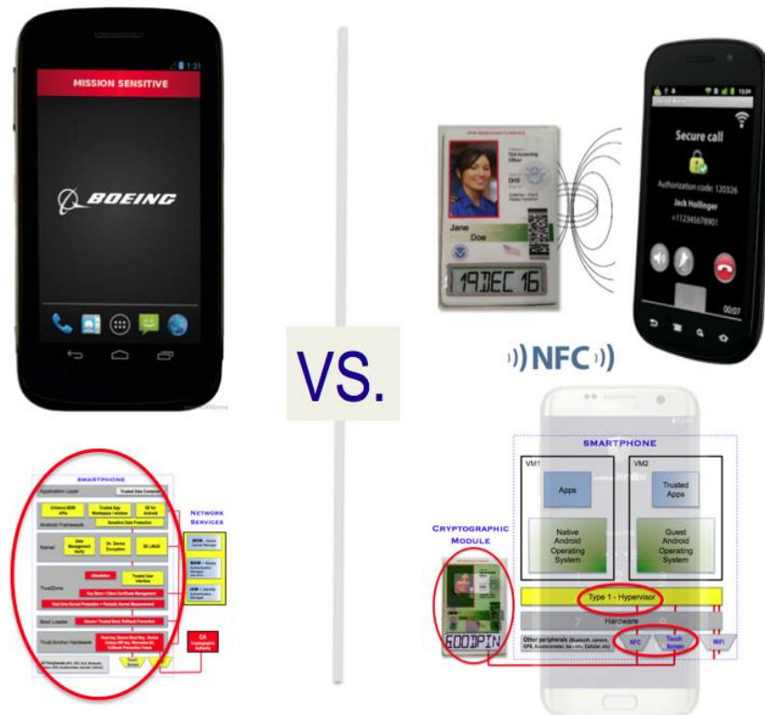
Figure 2 Comparison of a Full Custom Design Secure smartphone & functional block diagram to a Commercial smartphone tethered to a Tcreo NFC Cryptographic Module.
